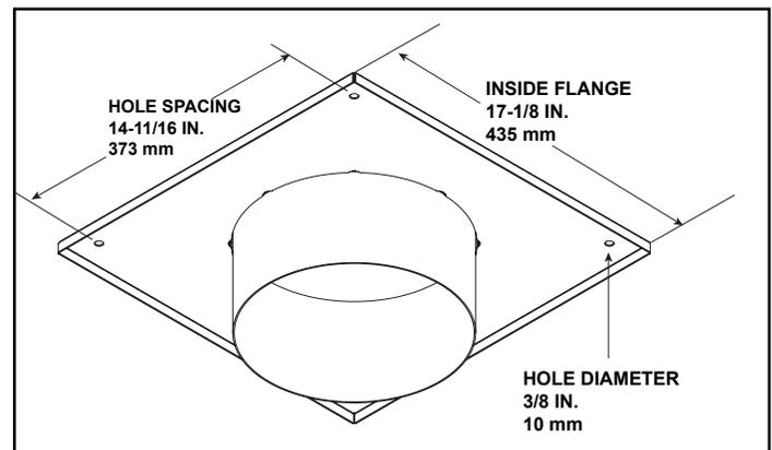
Figure 8D.2 10 Inch Chimney Collar Dimensions (RS14)
