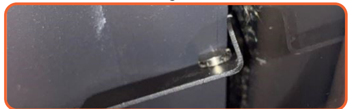
Figure 11.2 - Installing the screen tab
