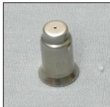
Figure 22: orifice de veilleuse
