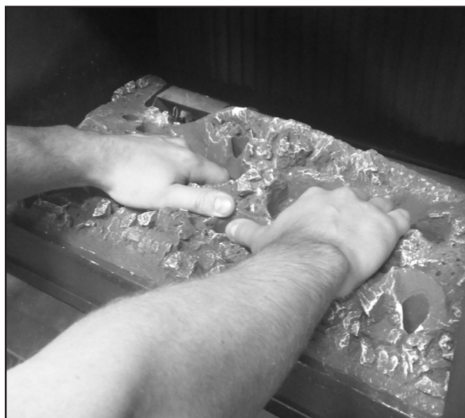
Figure 22. Burner Removal - Correct Hand Placement
