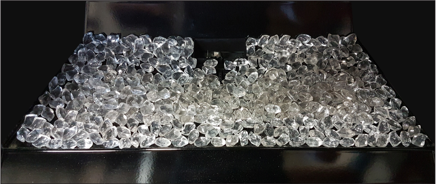
Figure 47: Burner tray with glass media installed.
