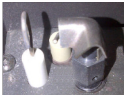
Figure 23: Proper Pilot Position
