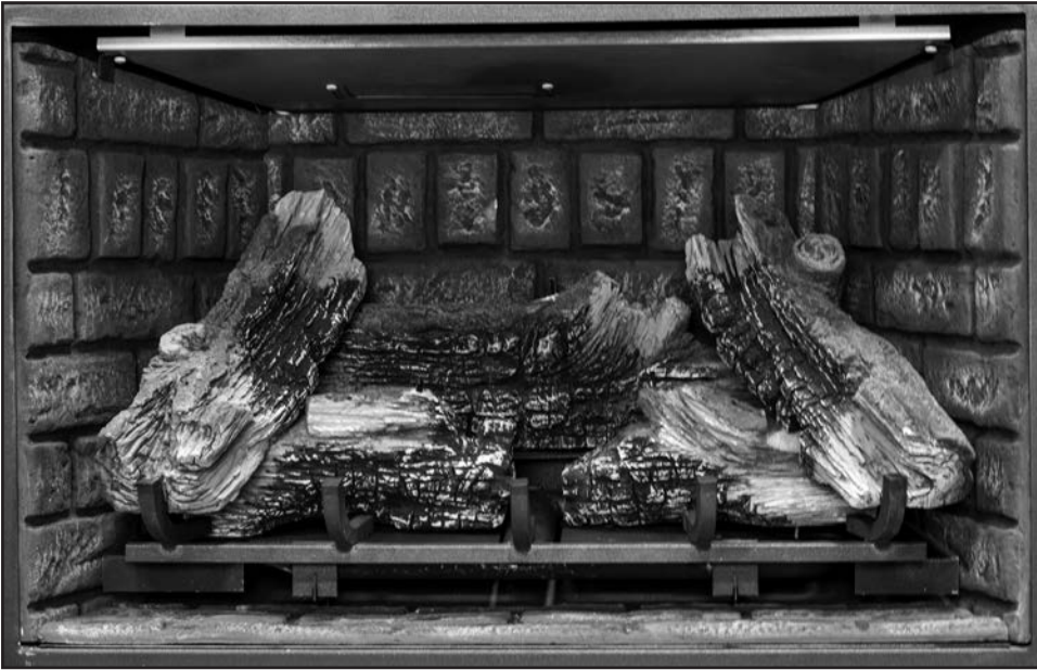
Figure 56: Install the right top log on top of rear log and right mid log. Locate the bottom on the far right grate arm.
