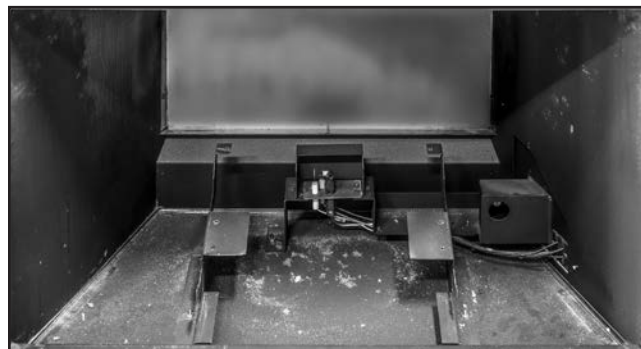
Figure 53: The rear liner can now be removed. Use a vacuum to clean up the bare firebox if needed.
