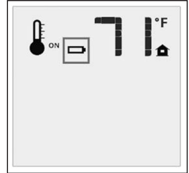
Figure 17: Low Battery Indicator.
