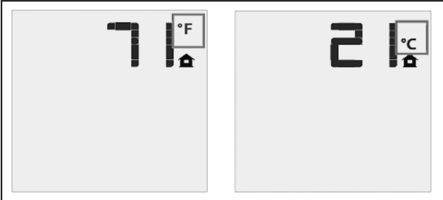
Figure 8: Thermostat Scale Display
