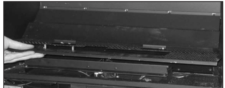
Figure 11: Removing Burner Tray.
