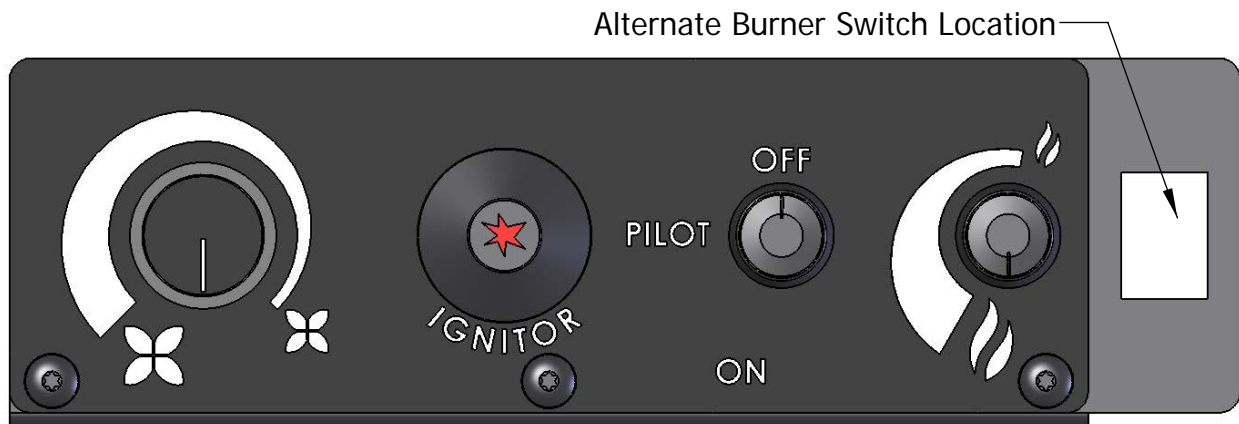
Figure 6: E20 Control Panel.
