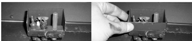
Figure 50: Pilot Shield Extension.
