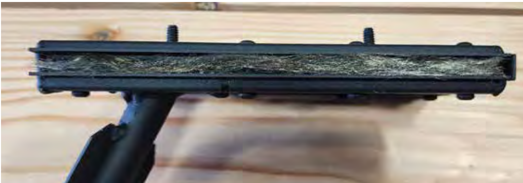
Figure 84: Nickel Strands Installed in Burner Slot
