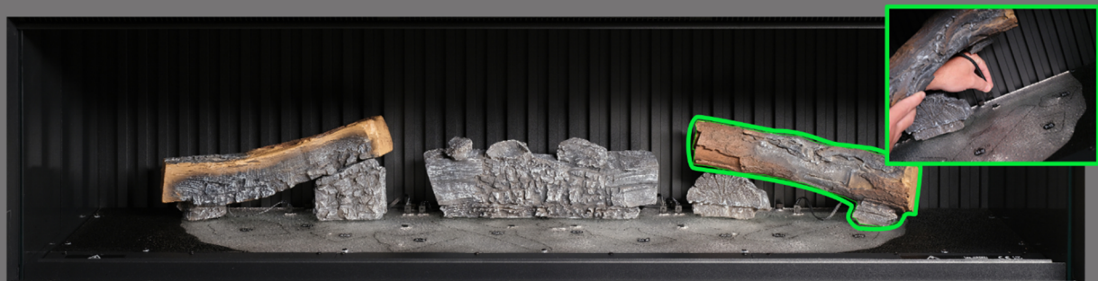
Step 6: Position log AI-3 onto the corresponding outline on the fuel bed, locating the peg on the underside of the log into the hole in the fuel bed, and plug the cable into the port on the fuel bed.
