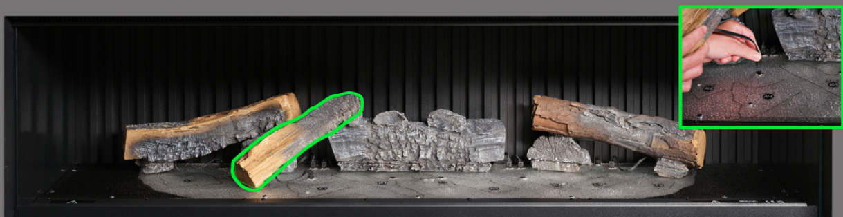
Step 7: Position log AI-9 onto the corresponding outline on the fuel bed, locating the peg on the underside of the log into the hole in the fuel bed, and plug the cable into the port on the fuel bed.
