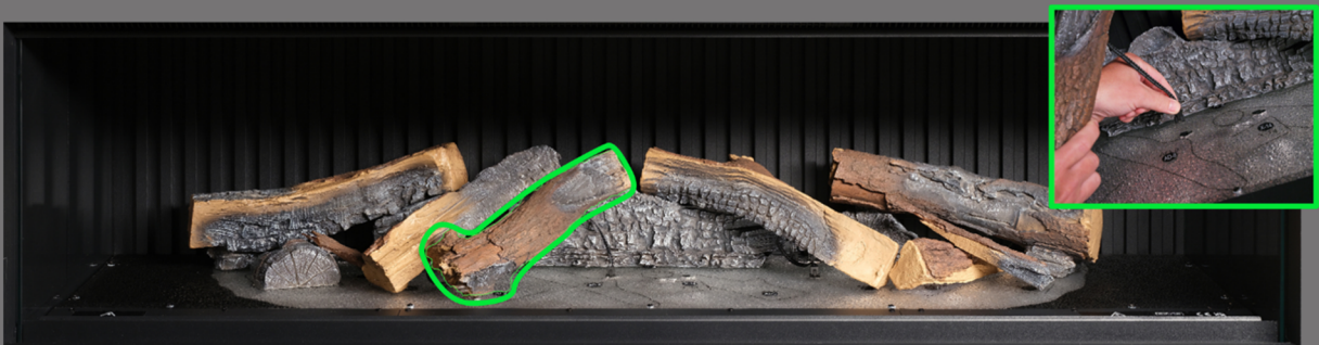
Step 13: Position log AI-4 onto the corresponding outline on the fuel bed, locating the peg on the underside of the log into the hole in the fuel bed, and plug the cable into the port on the fuel bed.
