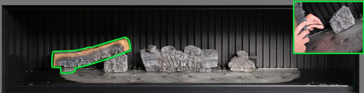
Step 5: Position log AI-1 onto the corresponding outline on the fuel bed, locating the peg on the underside of the log into the hole in the fuel bed, and plug the cable into the port on the fuel bed.
