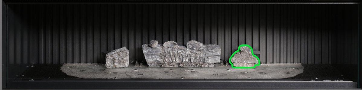
Step 4: Position log AI-8 onto the corresponding outline on the fuel bed, locating the peg on the underside of the log into the hole in the fuel bed.
