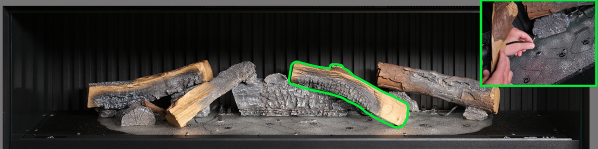
Step 10: Position log AI-6 onto the corresponding outline on the fuel bed, locating the peg on the underside of the log into the hole in the fuel bed, and plug the cable into the connector on the fuel bed.
