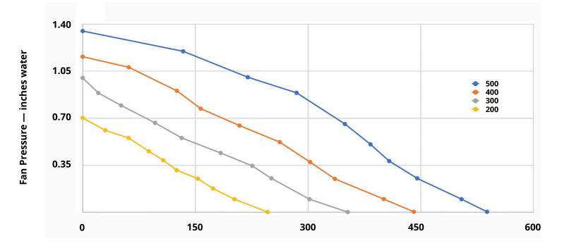
Fan Flow Rate — CFM Standard Air
