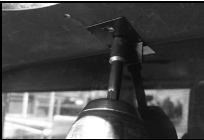
Figure 3 Retaining Bracket Installation - Back
