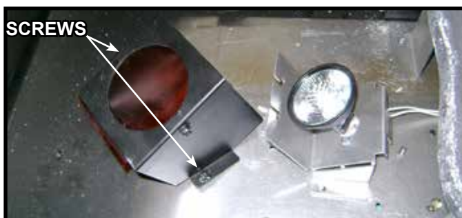
Figure 11.13 Light Housing Removed, Bulb Installed
