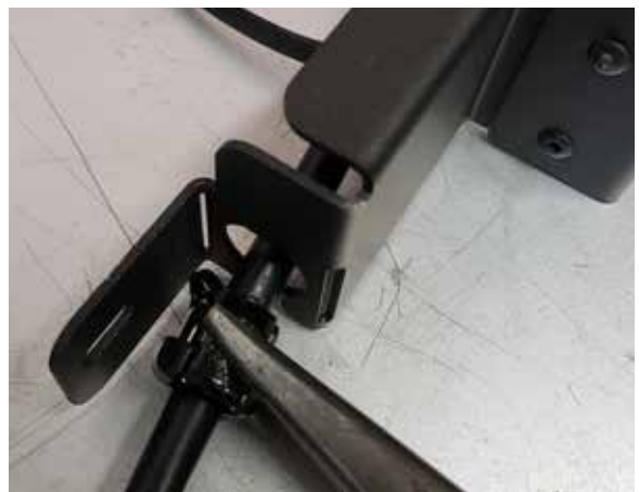
Figure 18: Left Strain install.
