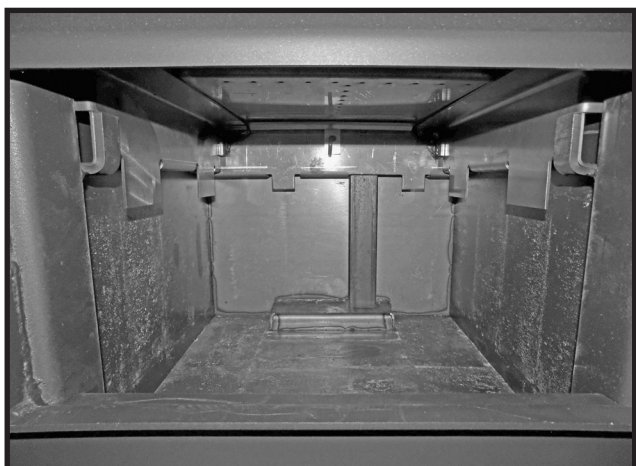
Figure 28: Chambre de combustion vide.
