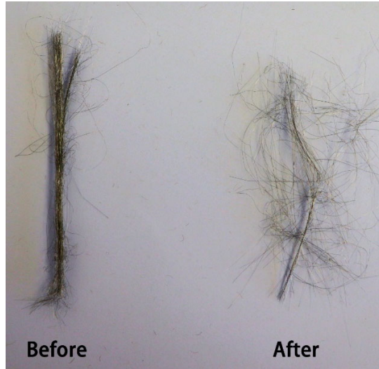
Left: Nickel strands as supplied | Right: Nickel strands ready to use
