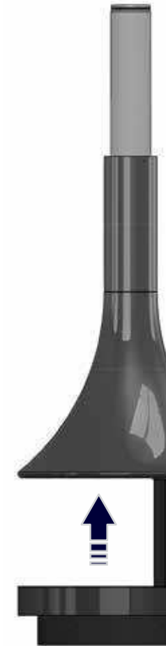
Raise the vent pipe back into place.
