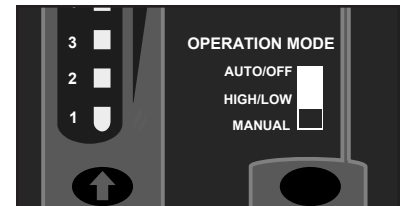
Figure 3: Thermostat Switch in MANUAL position.
