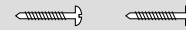
Two (2) No. 8 1½ in. (38 mm) round-head screws to securely attach the fan heater mounting bracket.
