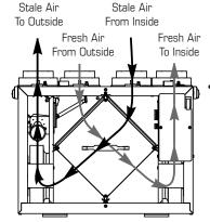
• 12" (305mm) of clearance in the front is recommended for removal of core
